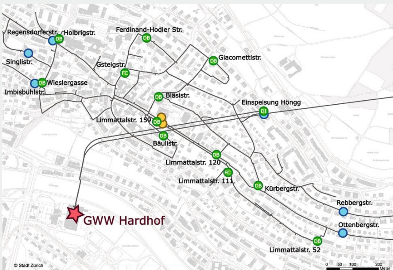
Fig. 1 Overview map of the sensor locations in the pilot area Höngg. The red star shows the Hardhof groundwater plant. The green dots refer to measuring points for quality measurements, the blue dots to measuring points for hydraulic measurements and the yellow dots to the two soil temperature measurements. The abbreviations in the green dots indicate the sensor type of the quality measurements. The main inflow into the pilot area is "Einspeisung Höngg" via the large supply line coming from the pumping station at Hardhof.
